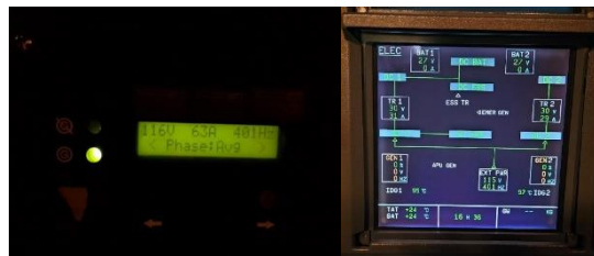
Figure 2. Aircraft electrical system When using GPU
