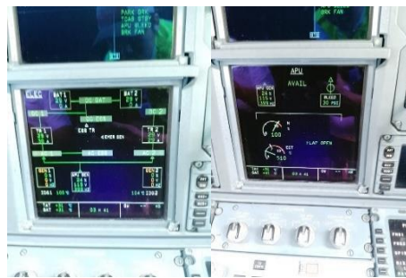
Figure 3. Aircraft electrical system When using APU
