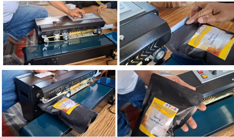
Gambar 3. Proses tahapan penggunaan mesin Continuous Band Sealer
