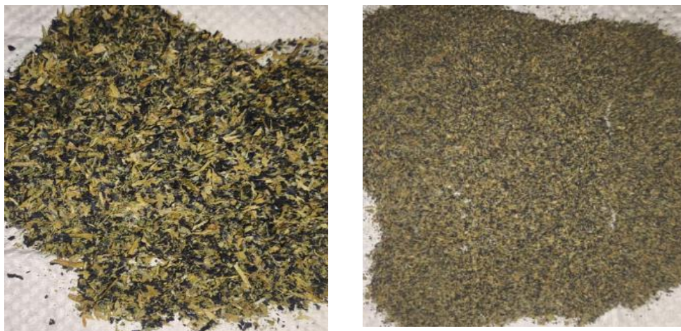
Figure 1. Appearance of Drying Using the Conventional Solar Heat Method for 3 days (a) and Food Dehydrator for 6 hours at a temperature of 60°C (b)
